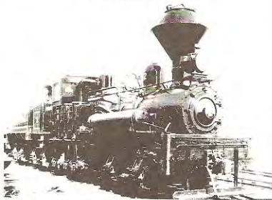
Early 1920s--Photo taken on arrival in Onalaska from dealer in Tacoma. The drive shaft was removed so that the engine could be towed.
